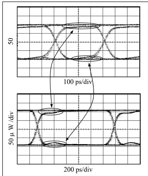
Figure 17. Eye Diagrams Showing Reflections at (a) 2.5 Gbps, (b) 800Mbps
