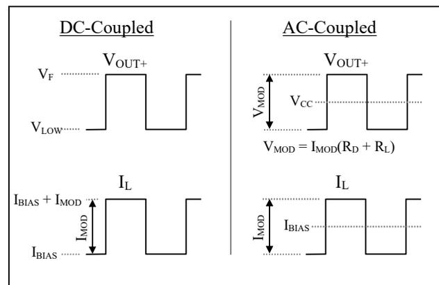
Figure 7. Output Voltage ( $V_{OUT+}$ ) and Laser Current ( $I_L$ ) for DC- and AC-Coupled Interface
