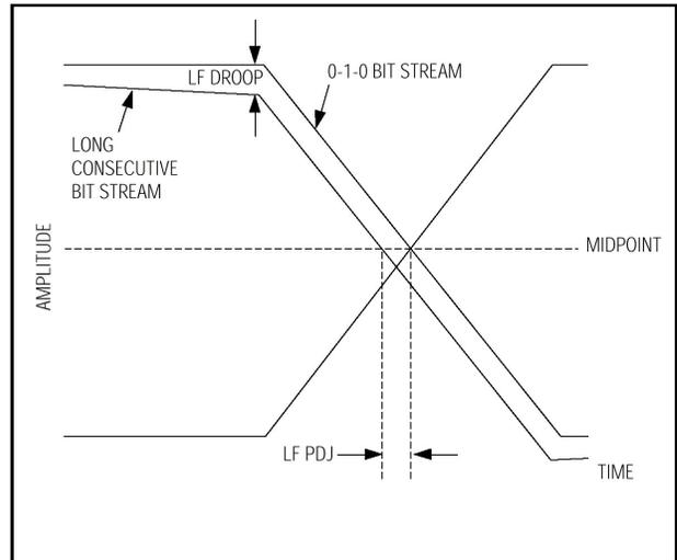
Figure 19. Pattern-Dependent Jitter Due to Low-Frequency Cutoff
