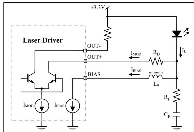
Figure 5. DC-Coupled Interface Circuit
