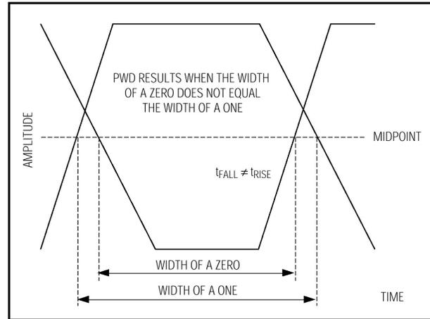
Figure 22. Pulse-Width Distortion
