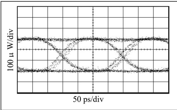
Figure 18. Eye Diagram Showing Double Line Pattern
