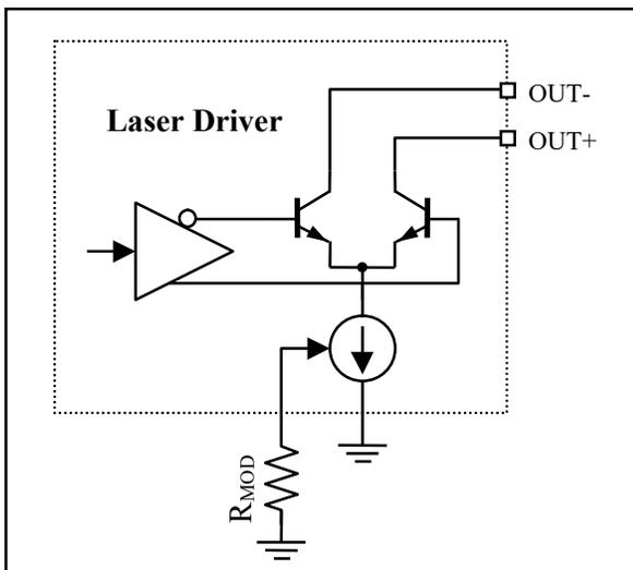
Figure 4. Typical Maxim Laser Driver Modulation Output Structure
