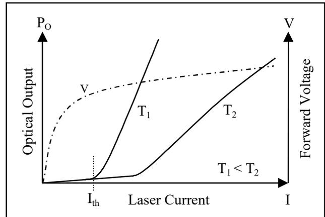
Figure 1. Laser Current, Forward Voltage and Optical Output
