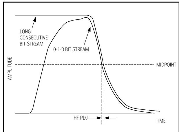
Figure 20. Pattern-Dependent Jitter Due to High-Frequency Rolloff
